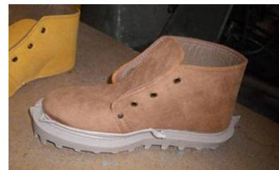
Similar considerations applied for the glued model, although the leather was resistant to the chemical nature of the glue formulation. In this case the good level of flexibility as demonstrated by the relative validation test in dry and wet condition assured the consistency of the leather grain and therefore, the firmness of the material (Figure 5.2.5).
