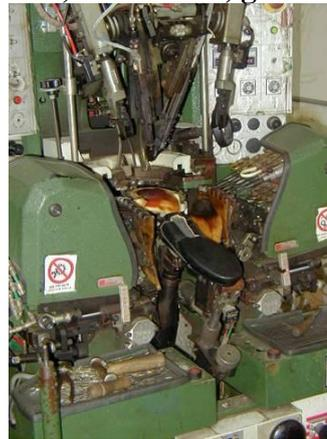
A particular note was drawn up for the models coming from the vulcanization, since the leather material was not affected by the high temperature procedure (120-135°C) which allowed the joining between leather and rubber. Although the shrink temperature of the leather was around 90°C, the short time required for vulcanization and the limited area of the leather subjected to it were not critical for the overall quality of the material (Figure 5.2.4).
