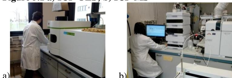
ICP-MS measurements were carried out with a quadrupole Agilent 7700 spectrometer, equipped with a collision cell system. Samples were introduced into the plasma by an auto sampler Agilent ASX-520. The instrument was fitted with a MicroMist Agilent standard nebulizer for 7700 and a Scott-type double-pass glass spray chamber cooled to 4°C. A solution of 10 µg/L of iridium in 2% HNO<sub>3</sub> was used as internal standard, according to the conditions of the instrument (**Table 5.1**).
